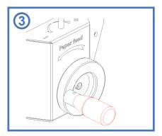
Turn the paper enter handle counterclockwise to make the honeycomb paper pass through the device.
